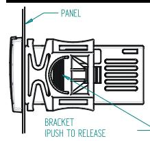
The instruments shall be mounted on vertical panel, in a 29x71 mm hole, and fixed using the special bracket supplied. The temperature range allowed for correct operation is 0÷60 °C. Avoid places subject to strong vibrations, corrosive gases, excessive dirt or humidity. The same recommendations apply to probes. Let air circulate by the cooling holes.
